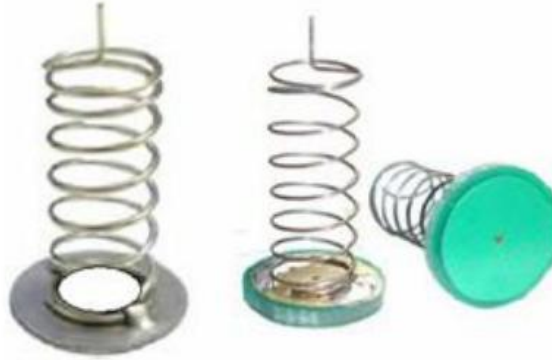
Figure 8: Spring sense element
