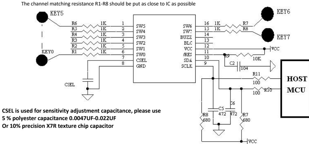
Figure 3: Working circuit diagram of WTC6508BSI
