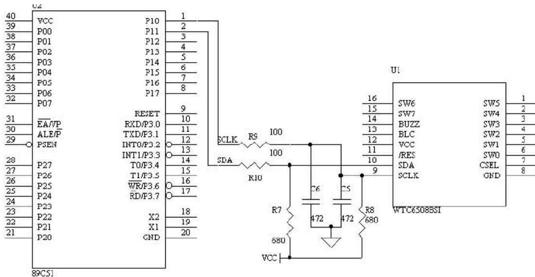
The corresponding circuit of the typical operating procedure
