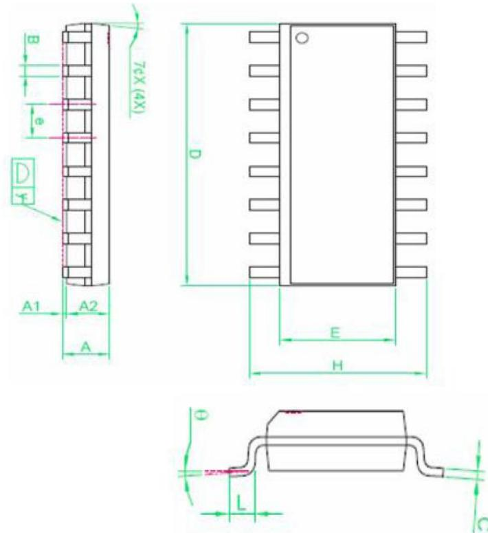
Figure 11: Package Dimension Drawing of WTC6508BSI
