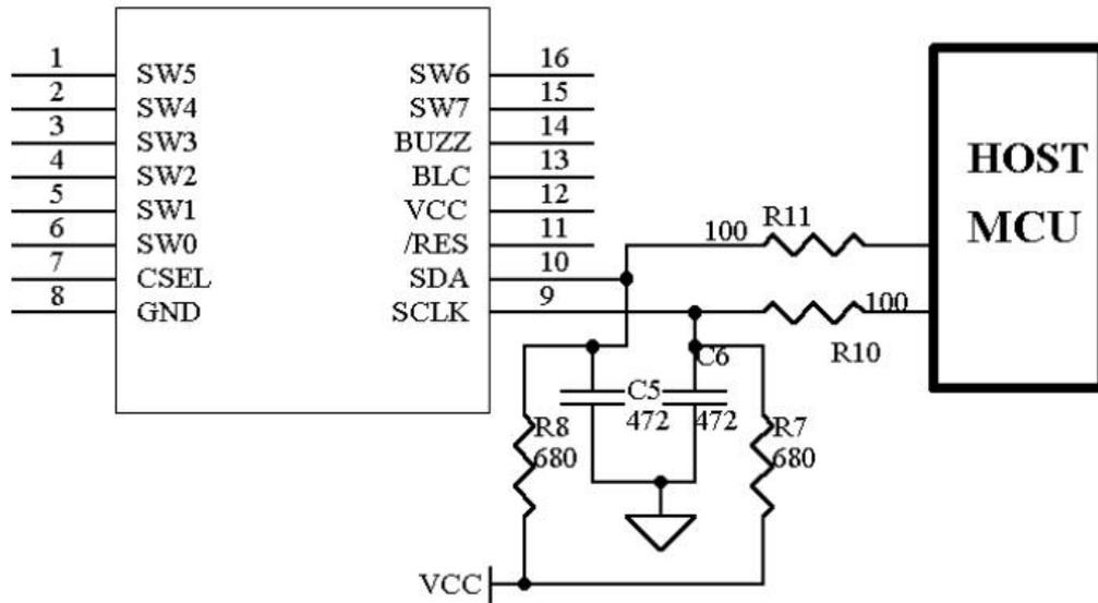
Figure 6: Serial interface circuit of MCU and WTC6508BSI
