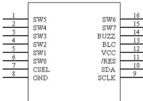
Figure 1: pin configuration diagram of WTC6508BSI
