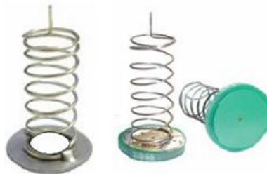
Figure 4: capacitance sensor made by metal spring (key sense element)
