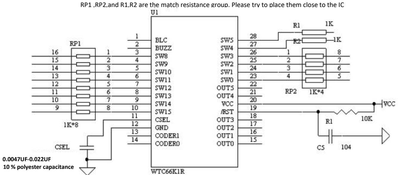
Figure 4: WTC66K1R Application Schematic Diagram
