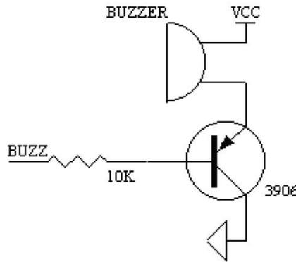
Figure 6: Buzzer drive electrical appliances
