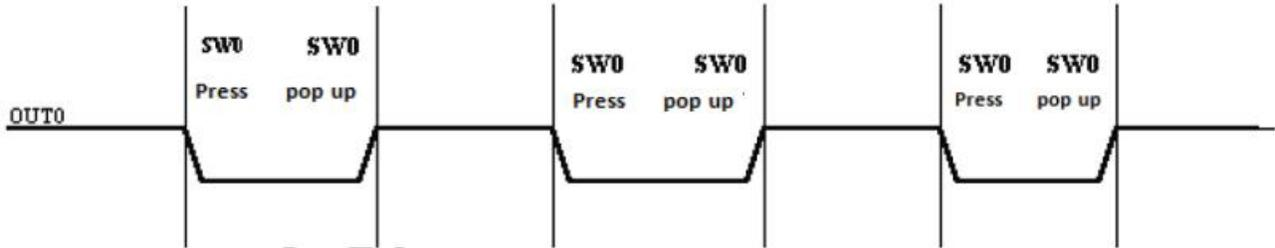
Figure 2: Sequence diagram of the output of the key
