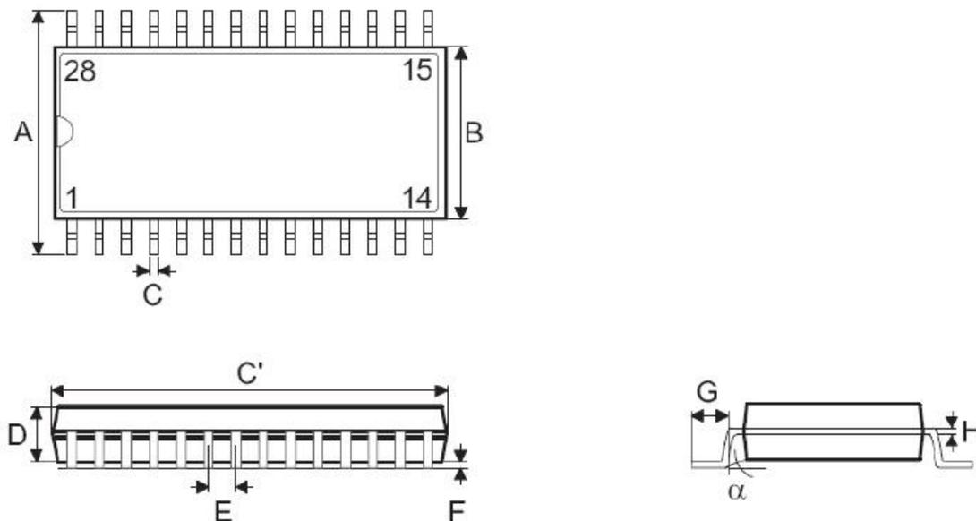
Figure 13: Package Dimension Drawing of WTC66K1R
