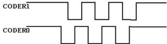
The anticlockwise rotation of the roller
