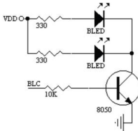
Figure 5: Backlight LED drive circuit
