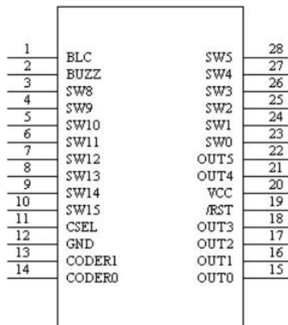
Figure 1: Pin Diagram of WTC66K1R
