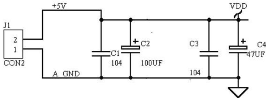
The analog and digital powers of circuit shall be connected separately to the ground in Y-connection method.
