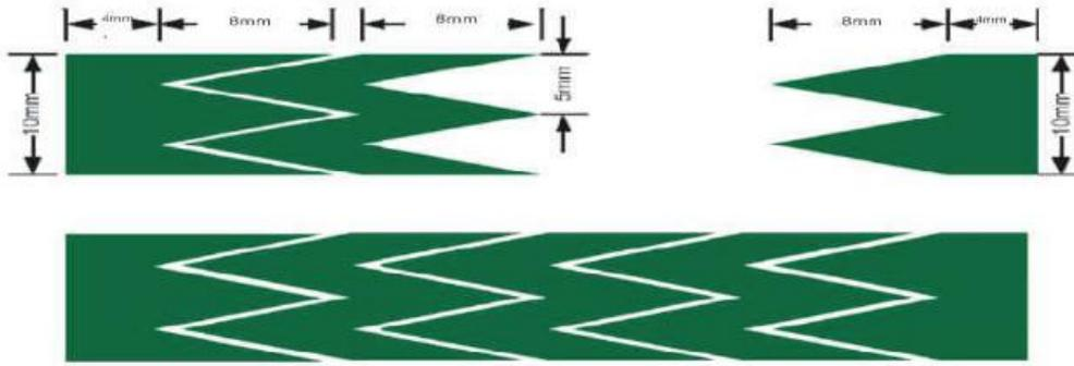
Figure 11: Geometry and dimension of touch slide bar
